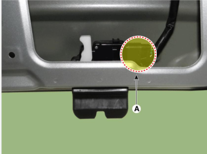
3. Remove the tailgate latch assembly after loosening the mounting bolts (A).
